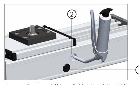
Lubrication is effected by an oiled felt insert. The felt can be re-oiled through lubrication nipples attached laterally to the ends of the roller packs.
